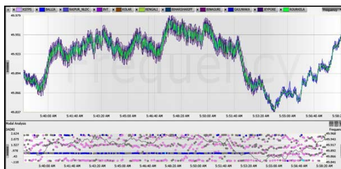
Figure 1. Zoomed view of Oscillation in frequency between 05:40- 05:59Hrs along with online Modal analysis.
