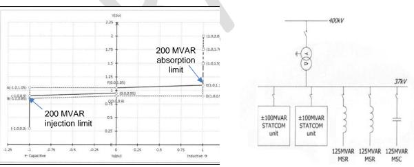
Figure 3: voltage and current output characteristics of 2 x 100Mvar STATCOM
