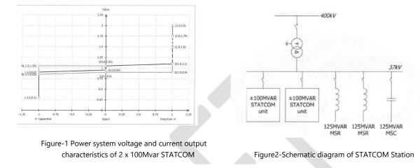
The STATCOM operates w.r.t Voltage on a slope with a dead band.
