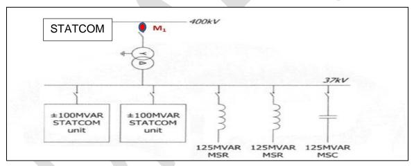
Figure 9: Schematic of Reactive Power Assessment at STATCOM
