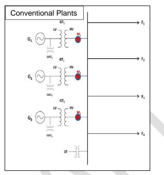
Figure 6: Schematic of Reactive Power Assessment at Conventional Plants
