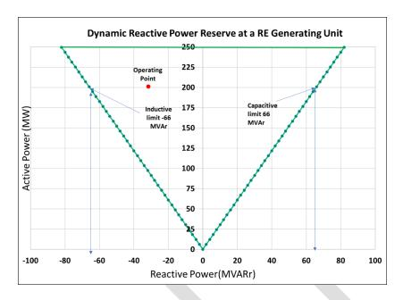
Figure 2: Reactive power limit of Inventor based Resources
