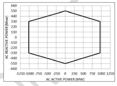
Figure 5: P-Q Capability curve of VSC Pugalur-Thrissur
