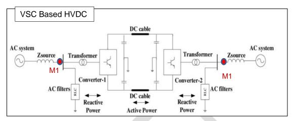
Figure 8: Schematic of Reactive Power Assessment at VSC based HVDC
