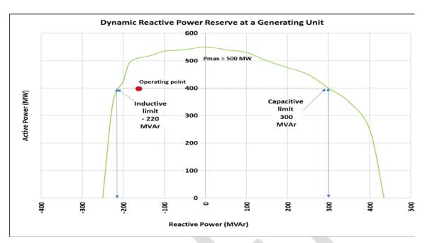
Figure 1: Reactive power limit of a Thermal Generating Unit
